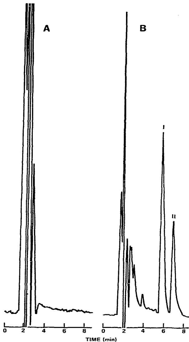
Fig. 3. Chromatograms of extracted patient plasma (A) not taking propafenone and (B) 1.5 h after taking 150 mg of propafenone orally. Peaks: I = propafenone; II = internal standard. The retention times of these two peaks are 5.9 and 7.0 min, respectively.
